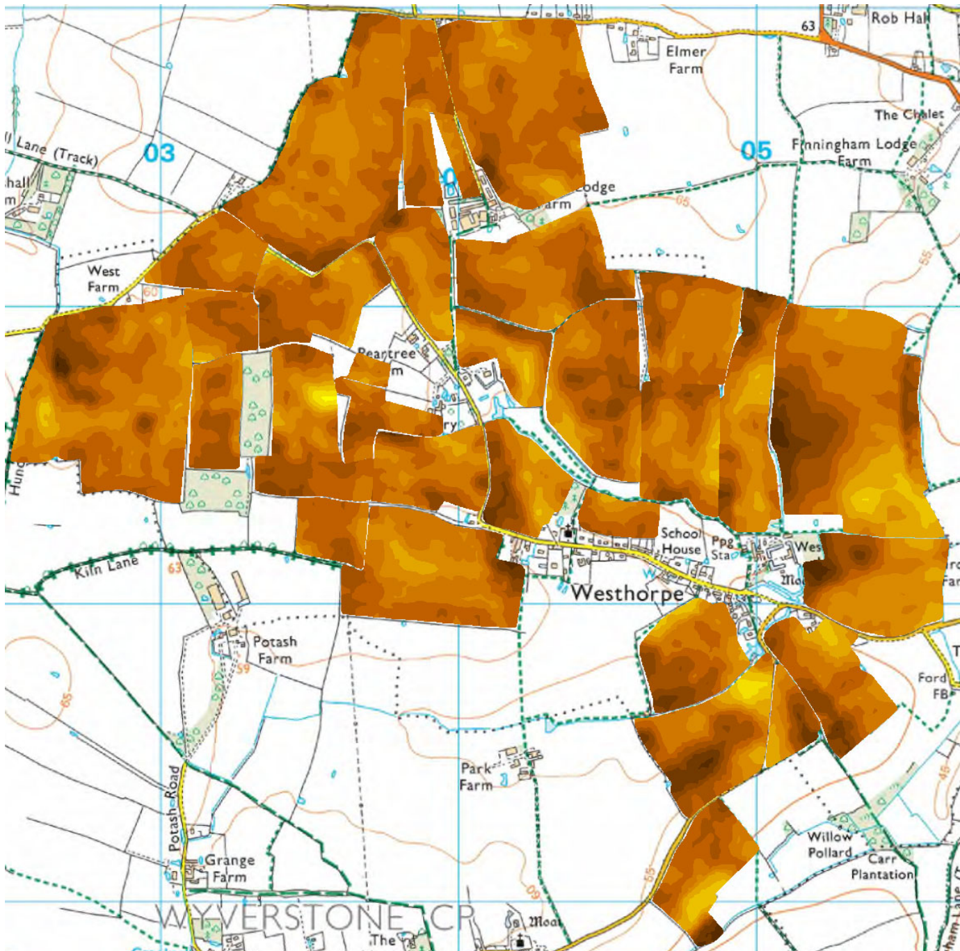
Figure 3 Shallow electrical conductivity (0 - 40 cm) measured in 2017 at Strategic Cereal Farm East
