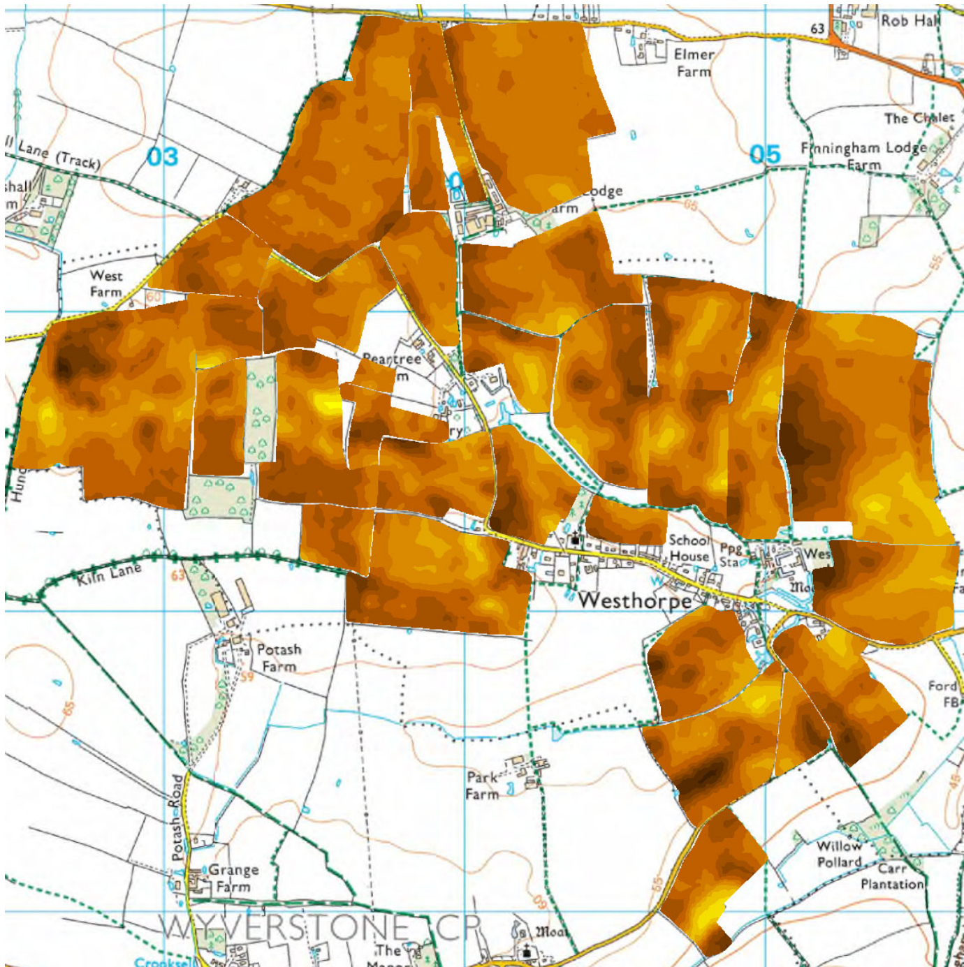
Figure 2 Deep electrical conductivity (0-120 cm) measured in 2017 at Strategic Cereal Farm East
