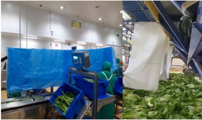
Figure 4. Examples of methods used to screen workers with plastic sheeting. Other methods could include solid Plexiglas screens
