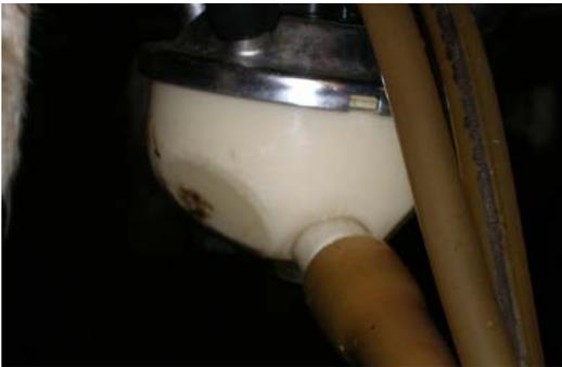
Figure 15. Blocked airbleeds
