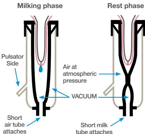
Figure 13. Teat cup vacuum and milk flow diagram
