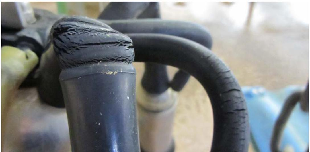
Figure 17. Badly cracked rubberwear
