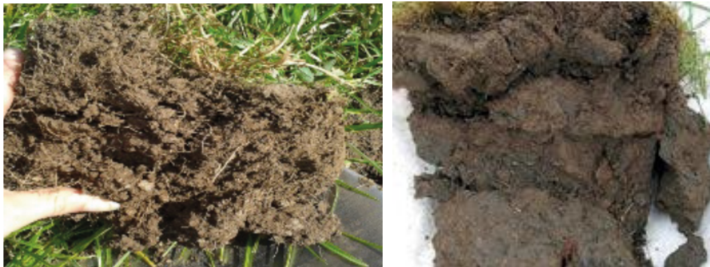
Figure 64. Soil compaction: Loose, friable soil (left); Compacted soil (right)
