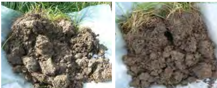
Figure 71. Soil structure from SRUC with machinery-compacted area with: sward lifting (left); surface aeration (right)
