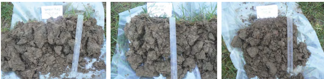
Figure 66. Soil profile following different compaction: Trampling compaction (left); Tractor compaction (middle); No compaction (right)
