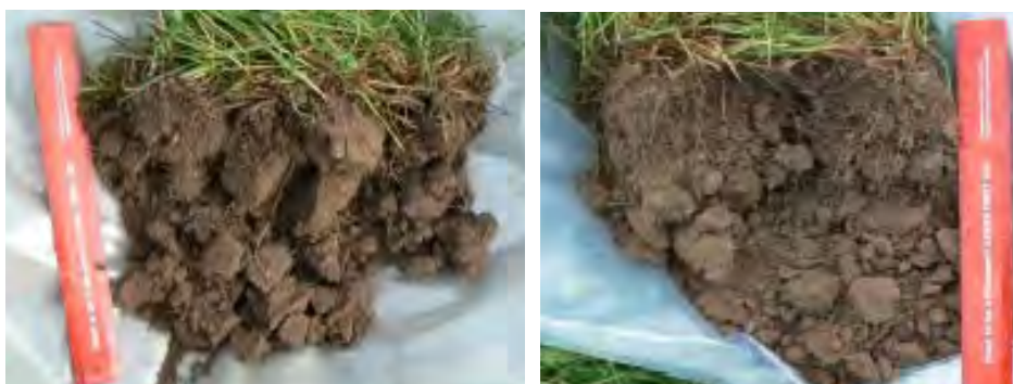
Figure 70. Soil structure from HAU: trampled area with no alleviation (left); trampled with surface alleviation (right)
