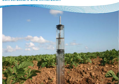
Figure 1. Mini Disk infiltrometer measuring effect of compost on soil infiltration
