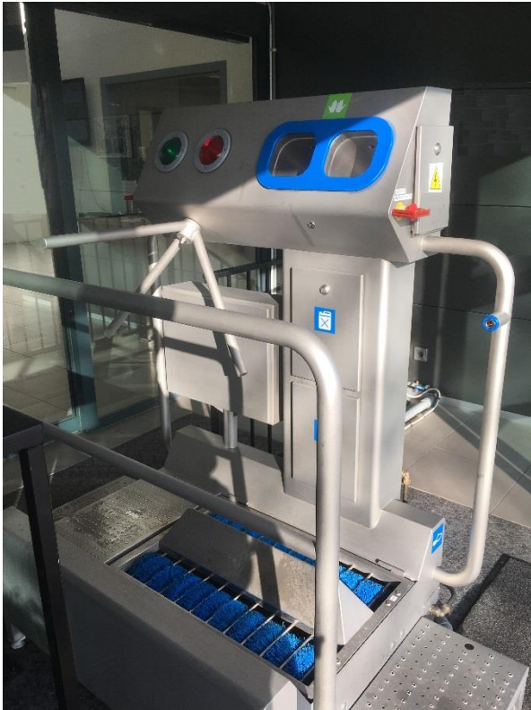
Figure 2. Hygiene lock at the entrance/exit of a propagator in the Netherlands – image with permission of the propagator.
