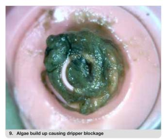
For the smaller particles which are very problematic for blocking the nozzles of drip irrigation systems, **fast sand filters**, **disc filters** or **screen filters** are employed.
