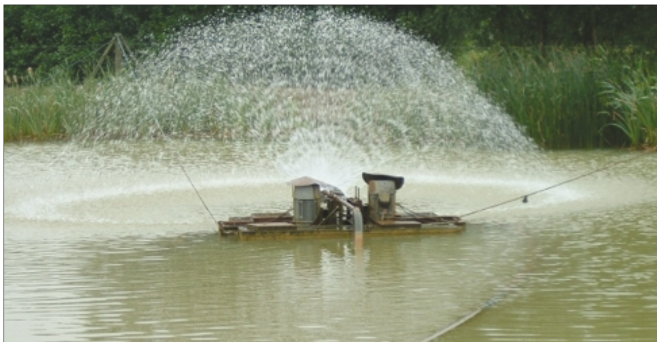
4 High levels of iron in water intended for irrigation purposes, can be lowered by aerating it
