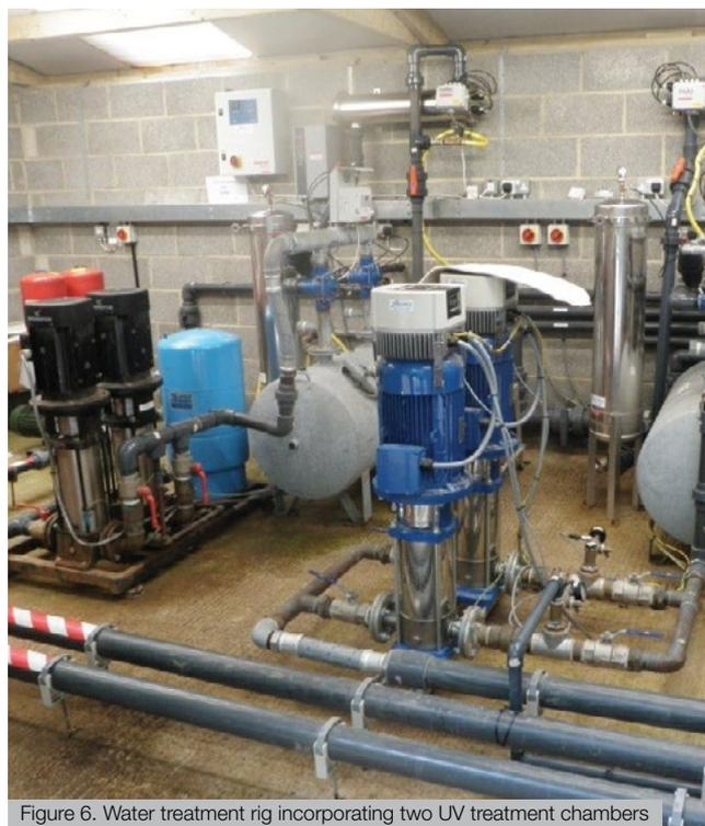
Figure 6. Water treatment rig incorporating two UV treatment chambers
