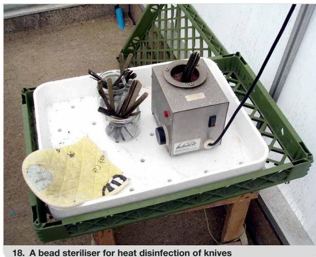
18. A bead steriliser for heat disinfection of knives
