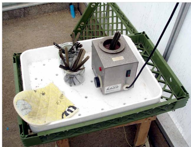
18. A bead steriliser for heat disinfection of knives
