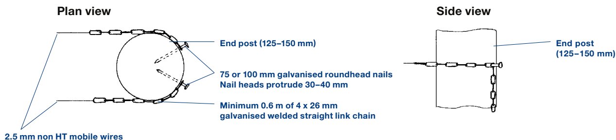
Diagram 5 Method of holding chains on end posts with single bolt
