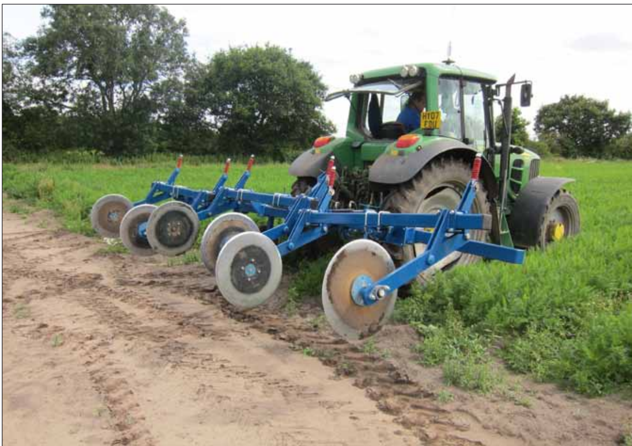
8 Machinery designed to clip the foliage from the edge of the carrot bed
