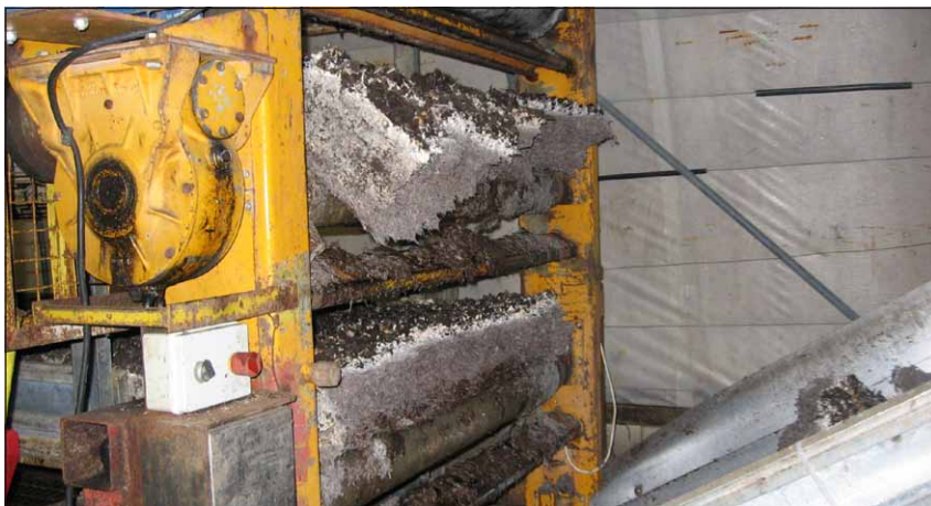
11 Spent mushroom compost is removed in lumps
