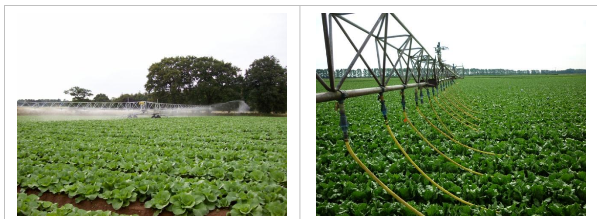
Figure 4 Hosereel fitted with (a) boom and (b) modified with drop tubes on lettuce in Cambridge, UK (2012).
