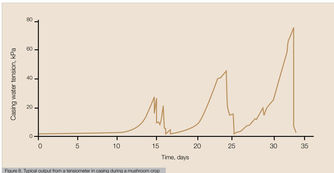
Figure 8. Typical output from a tensiometer in casing during a mushroom crop
