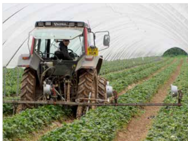
19. Some growers use tractor mounted applicators to introduce bulk quantities of predatory insects
