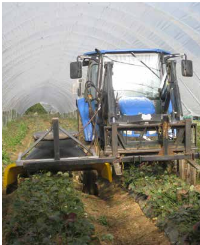
11. Front mounted bug vacuum can successfully reduce numbers of European tarnished plant bug in strawberries
