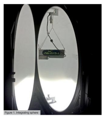
In project CP 139 a 1.8m integrating sphere at the Lighting Industry Association (LIA) laboratories in Telford was used to measure the spectral performance of a range of lights. Also a 7m goniometer at Piseo in France was used to measure the performance of the accompanying luminaires.
