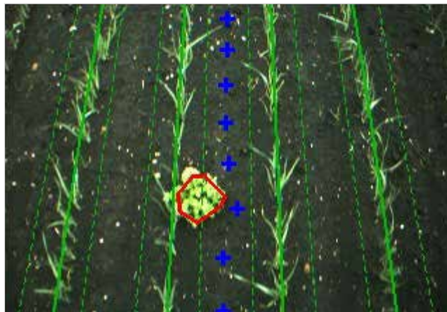
3. Screen shot of the machine console when operating in leeks showing row crop tracking information and a large broadleaf weed that the system has detected and marked with a red outline
