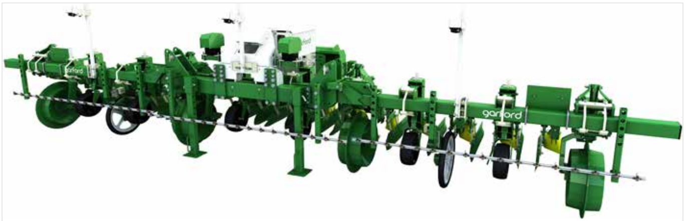
2. A hooded band sprayer equipped with a spot spray bar and three cameras
