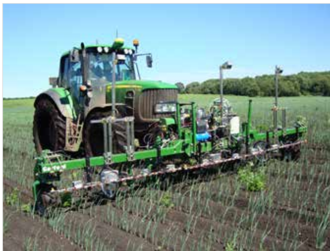
4. Experimental prototype machine operating in a crop of leeks to treat mugwort
