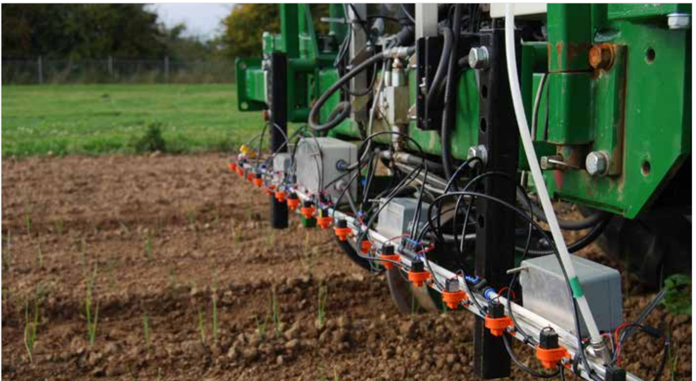
1. The new herbicide spot sprayer system developed in HDC HortLink project FV 307a
