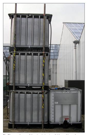
Bio-filters can be a useful system to treat pesticide washings where space is a limiting factor
