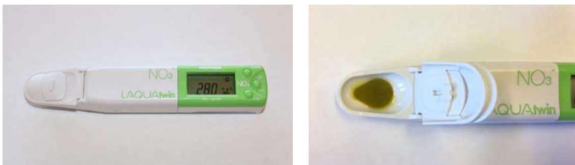
Fig. 1: LAQUAtwin nitrate electrode (figure on the left) and flat sensor of the LAQUAtwin nitrate electrode filled with sample fluid
