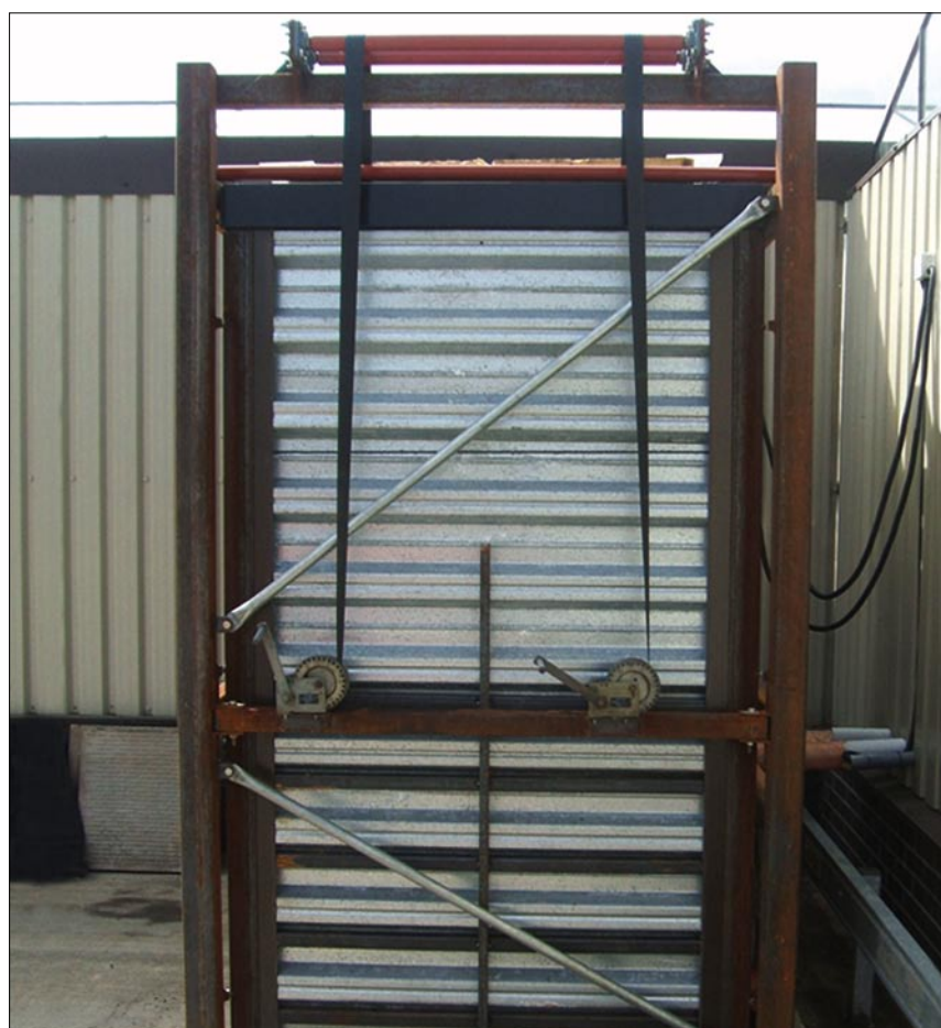
4 Side view of tank showing winding mechanism used to lower platform and crate into tank. Crates are placed on the platform using a forklift truck
