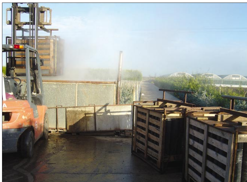
2 Crates being lowered into hot water tank by forklift truck
