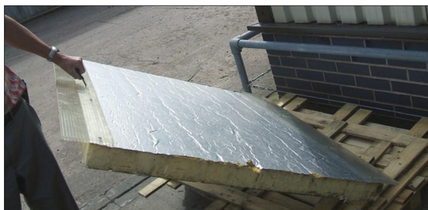
5 Typical insulated tank lid to reduce heat loss and water evaporation
