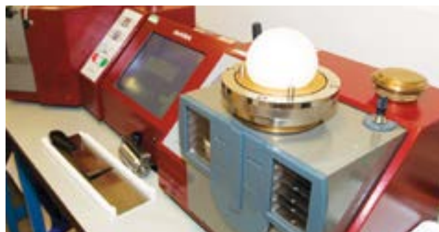
Chopin Alveograph showing stage 5 – air being pumped into dough.
