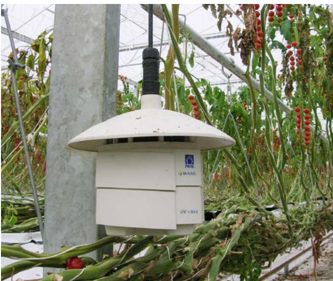
Figure 25. Measuring box incorporating an electronic humidity sensor
