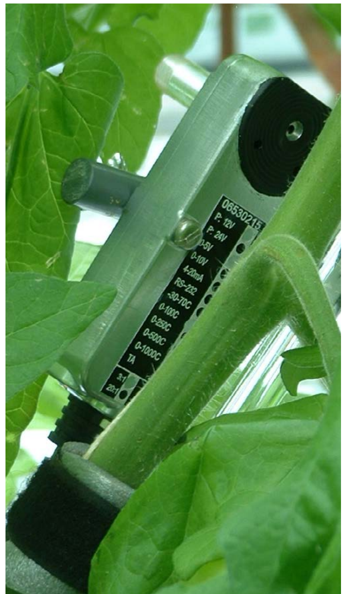
Figure 29. Infrared sensor used to measure plant or plant organ temperature
