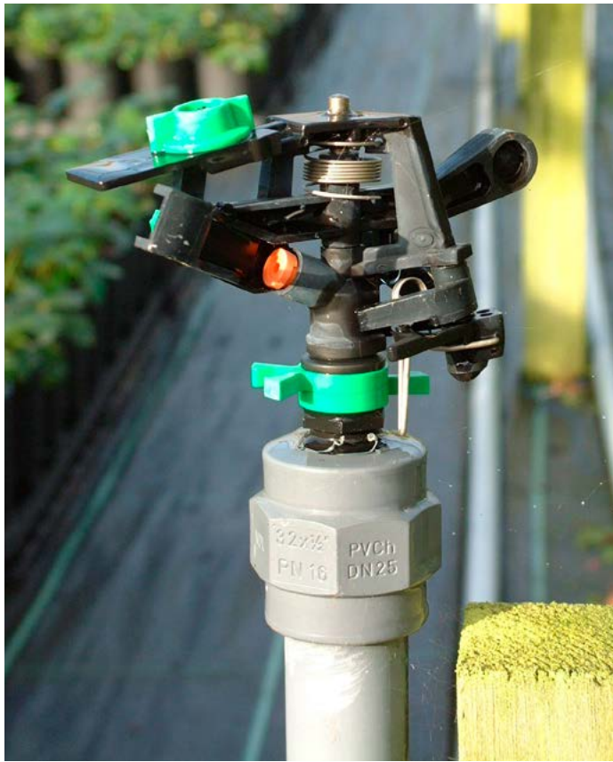
Figure 13. Setting part-circle impact sprinklers to a 220° arc down the sides of beds will usually improve wetting of edge containers compared to a 180° arc
