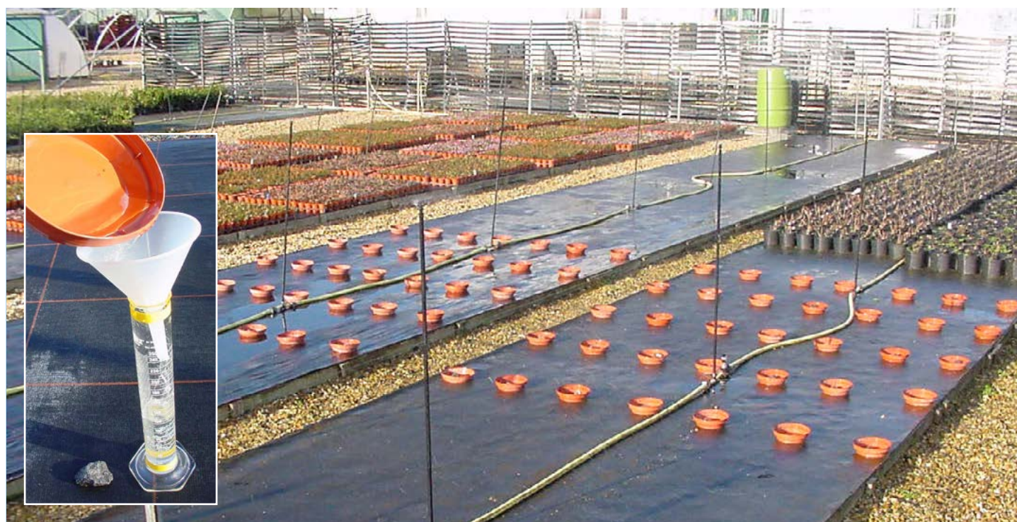
Figure 4. The use of equidistantly spaced saucers over a representative bed area for measuring irrigation output and distribution
