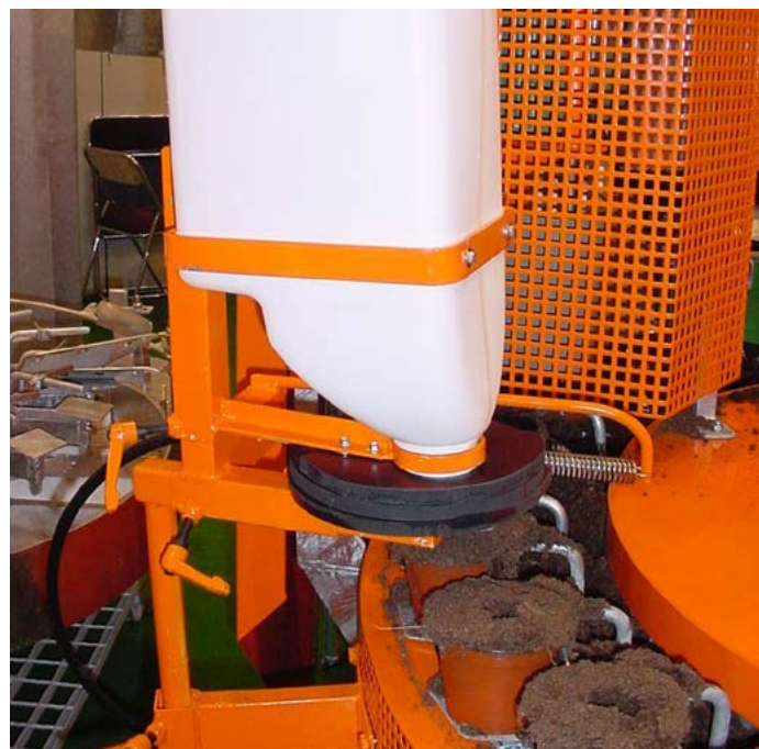
Figure 5. A CRF dispenser can deliver a measured amount of fertiliser into the base of the drilled planting hole when machine potting
