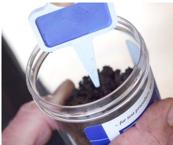
Figure 5. The Solvita® soil health test measures the carbon dioxide evolved from respiration of soil organisms
