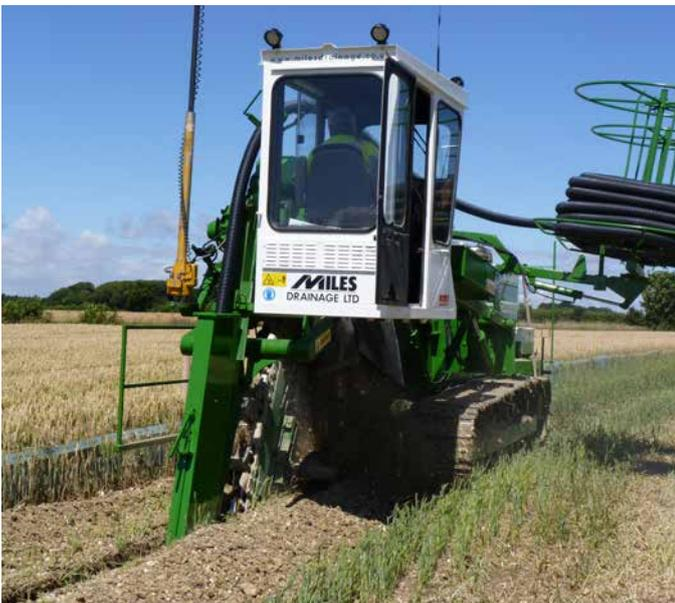
Figure 31. Installing land drains with laser gradient control
