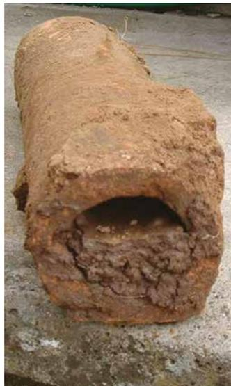
Figure 22. Silted clay drain
