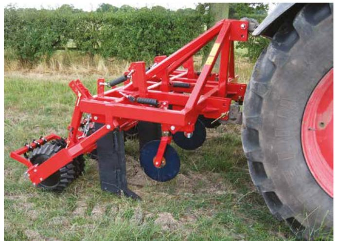
Figure 11. Topsoil loosener for grassland
