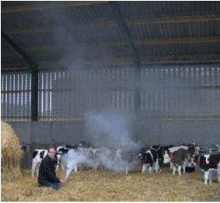
Use a smoke test to show the flow of air within a building
