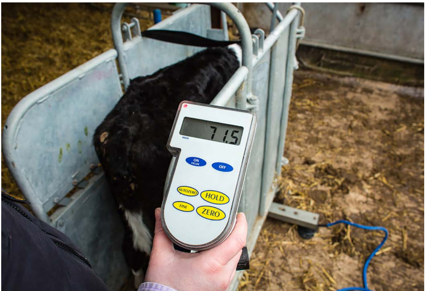
Figure 17. The most accurate way to weigh calves is to use a set of electronic weigh bars
