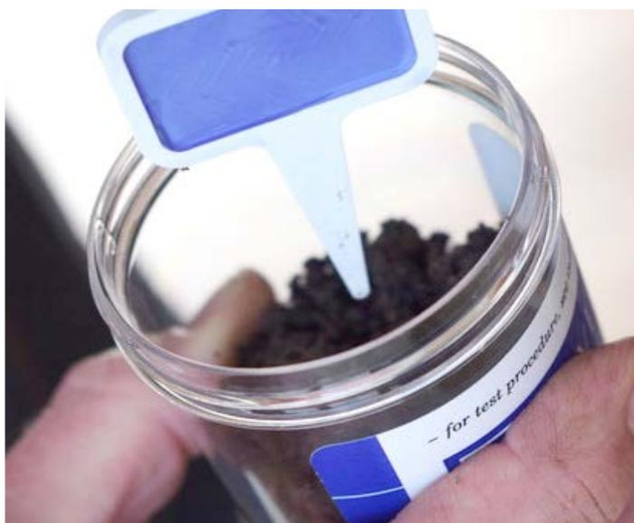
Figure 2. The Solvita® soil health test measures the carbon dioxide evolved from respiration of soil organisms
