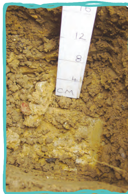
Compacted layer at 15cm.
