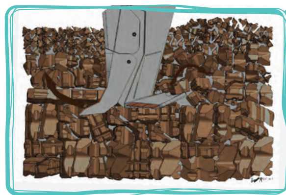
A winged subsoiler tine at 'effective working depth' just below the compacted layer loosening the soil.
