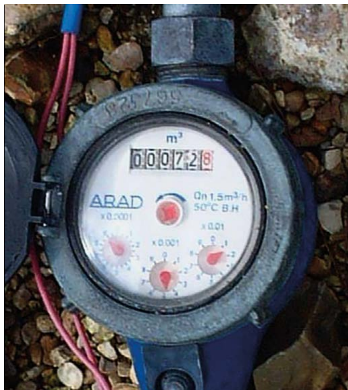
Figure 2. Using meters to record total water volumes used for all or part of the nursery is a useful tool for effective water management. This water meter is reading 72.8159m 3 or 72,816 litres
