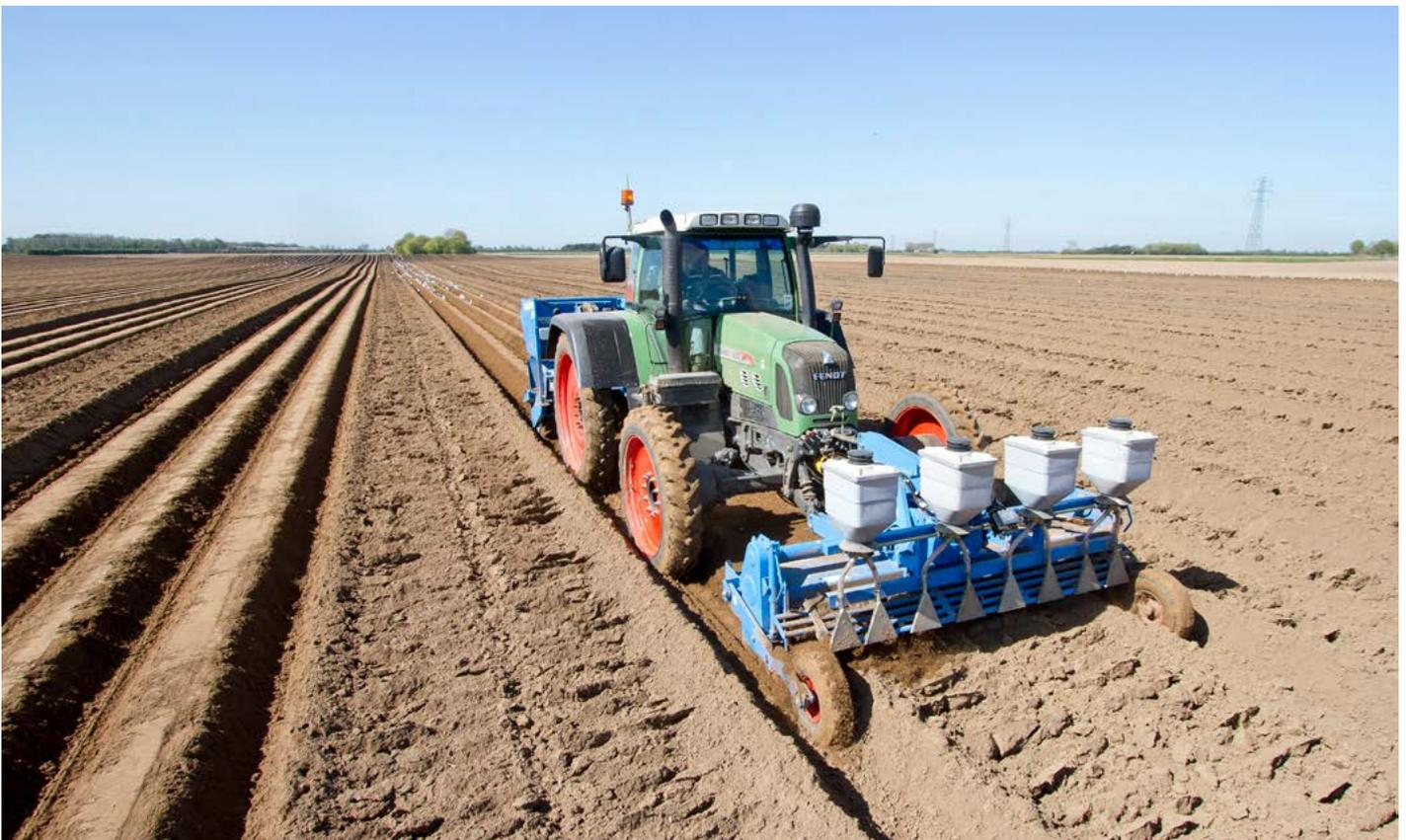
Figure 22. Nematicide applicator and rotavator on the front of a tractor pulling a planter
