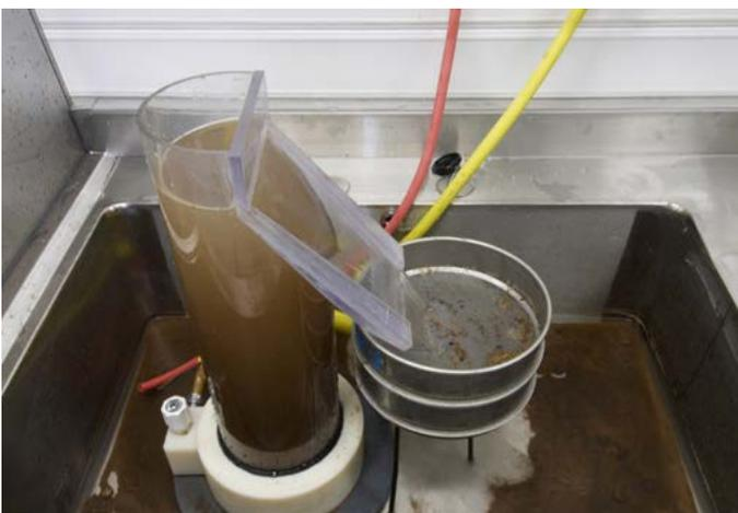
Figure 15. Wye washer, an elutriator for extraction of cyst nematodes from wet soil.
