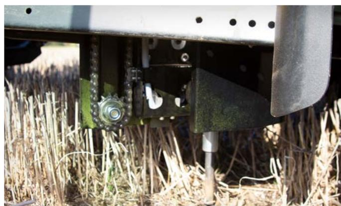
Figure 12. Soil sampling machine attached to field vehicle
