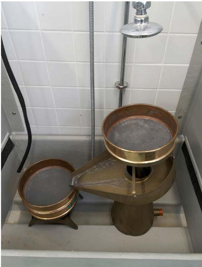
Figure 14. Fenwick can, in use to extract cyst nematodes from wet soil.
