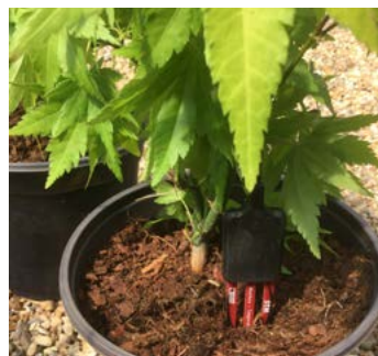
Figure 7. Examples of various growing media moisture sensors (note some have been lifted from the media to show the various designs available)
