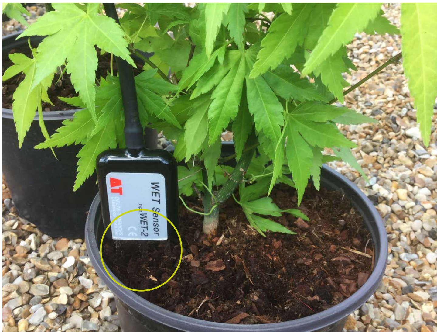
Figure 10. Example of poor sensor positioning – the probes are proud of the medium and the sensor is too close to the container rim which will lead to erroneously low readings
