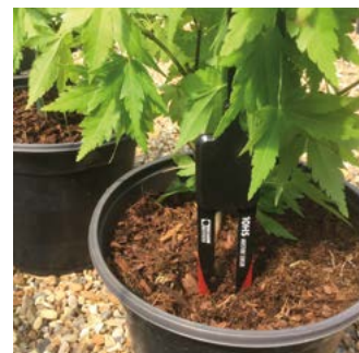
Figure 7. Examples of various growing media moisture sensors (note some have been lifted from the media to show the various designs available)
