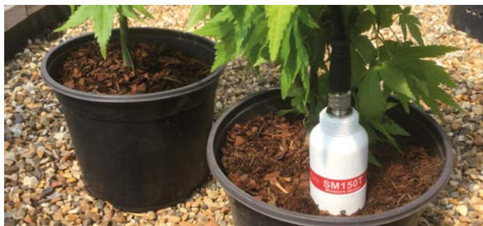
Figure 7. Examples of various growing media moisture sensors (note some have been lifted from the media to show the various designs available)
