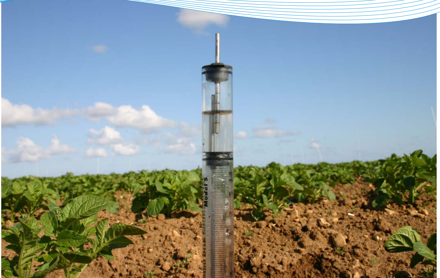
Figure 1. Mini Disk Infiltrometer measuring effect of compost on soil infiltration
