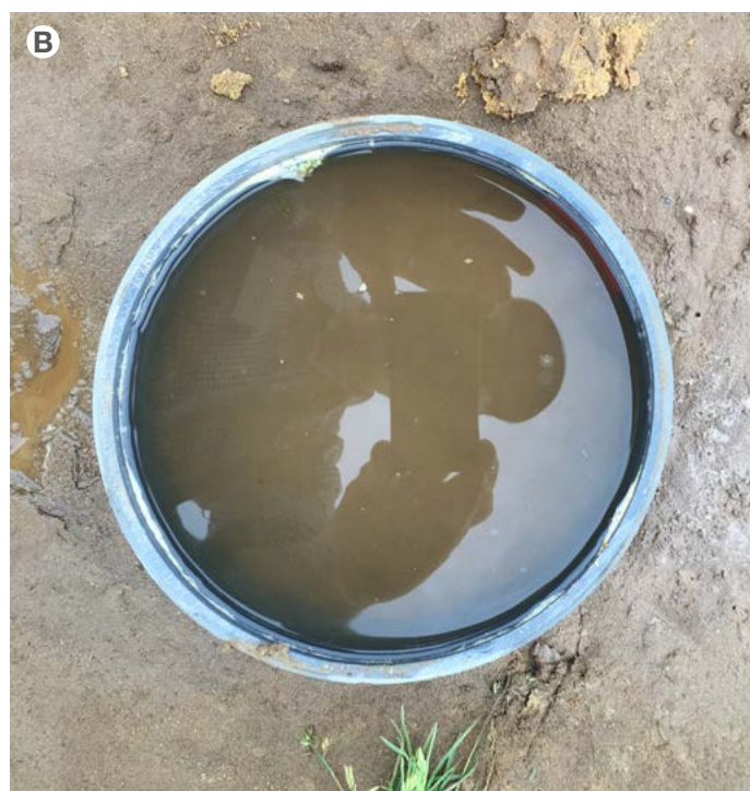
Figure 2. Simple infiltrometer using drainpipe to demonstrate difference between A) good infiltration in a bed used to grow coriander, and B) poor infiltration in the adjacent wheeling
