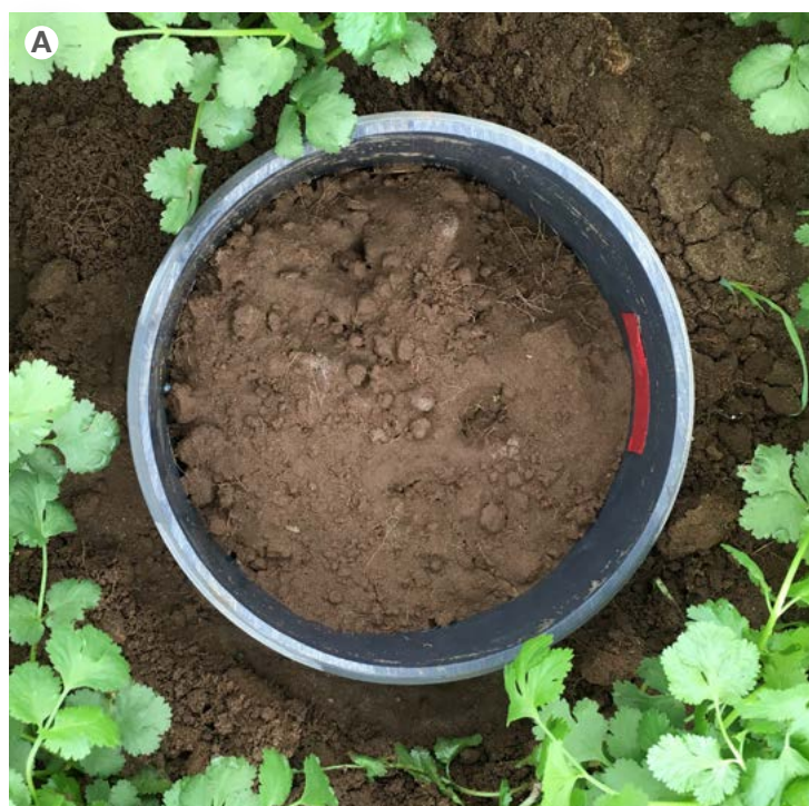
Figure 2. Simple infiltrometer using drainpipe to demonstrate difference between A) good infiltration in a bed used to grow coriander, and B) poor infiltration in the adjacent wheeling
