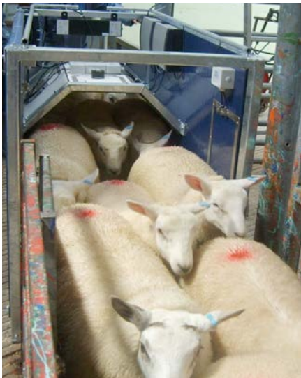
Figure 5. Example of an EID race reader for sheep
