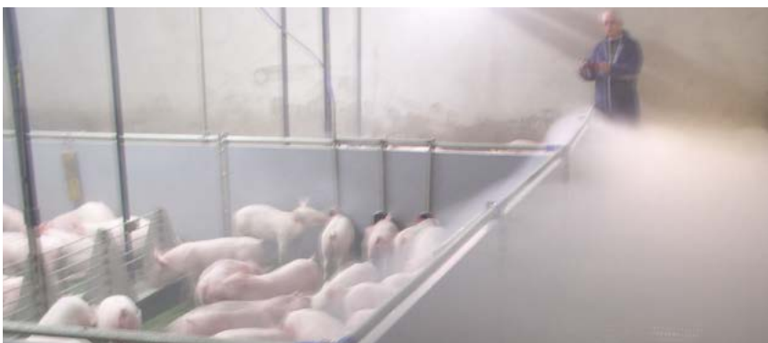
Figure 35. Smoke test showing air moving upwards from low-level inlets and over the solid pen wall
