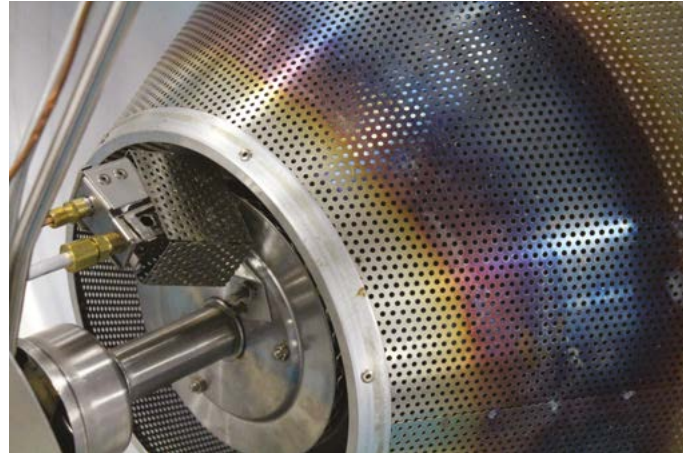
Figure 60. Gas radiant burner
