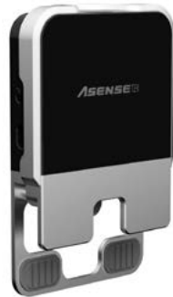
Figure 11. The Asense Lighting Passport, a 'smart' light meter
