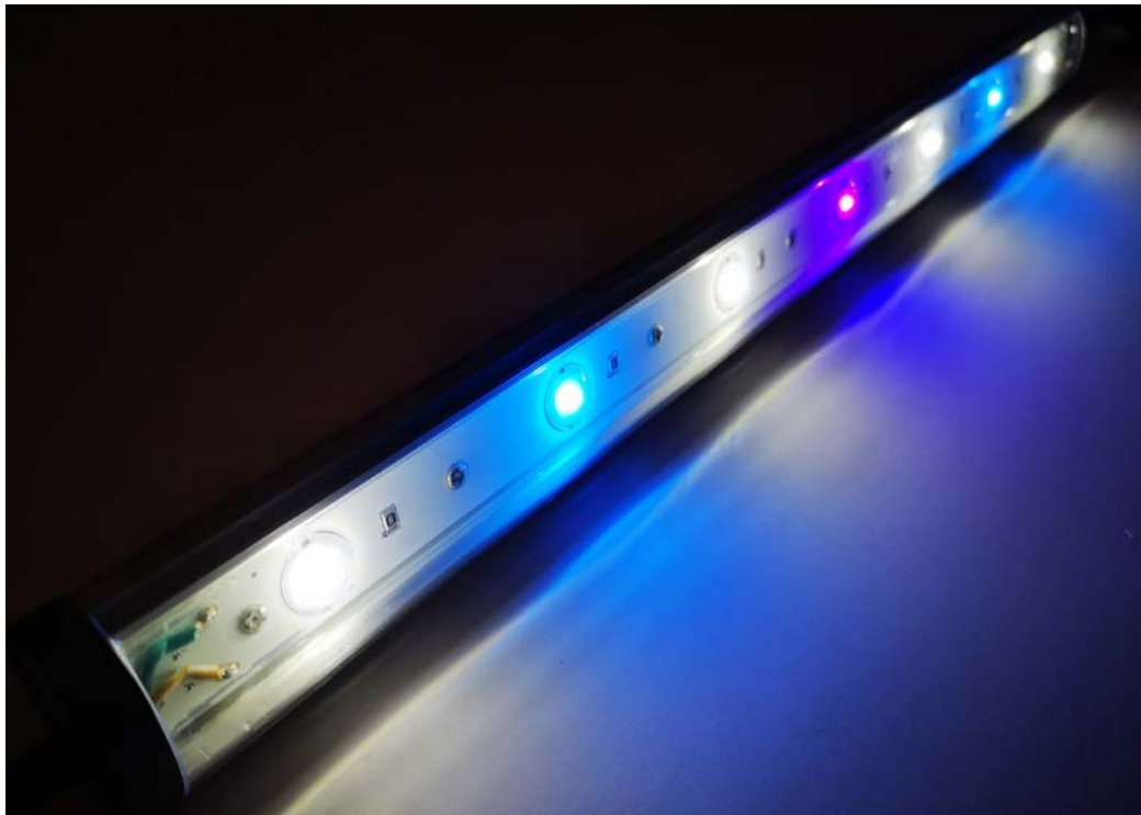
Figure 4. Biolumen Ltd 500 strip, an LED strip light producing blue, white and near-UV light for pigs
