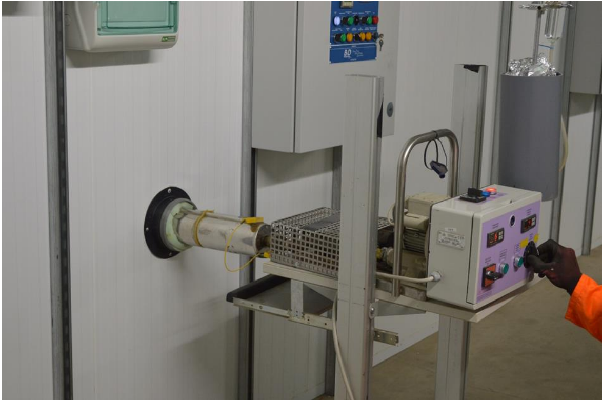
Fig. 2. CEDAX Electrofog EWH-3000 for application of spearmint oil and DMN.
