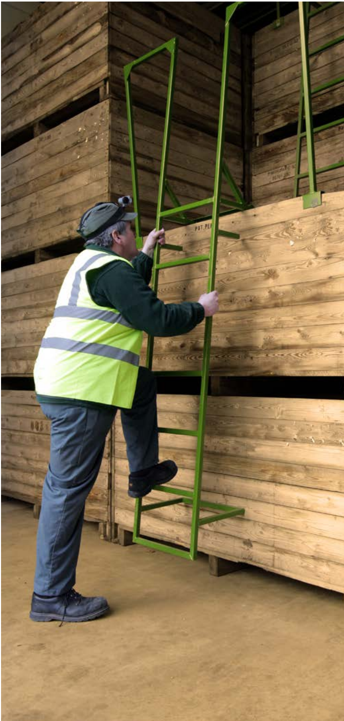
Figure 34. Working at height on stepped ladders in a box store
