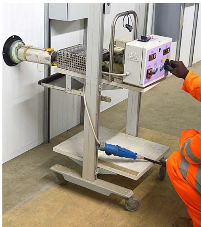
Figure 29. Hot fog application of sprout suppressant using an electrical fogger
