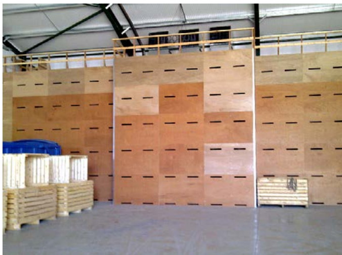
Figure 15. Open suction is a non-positive drying solution
