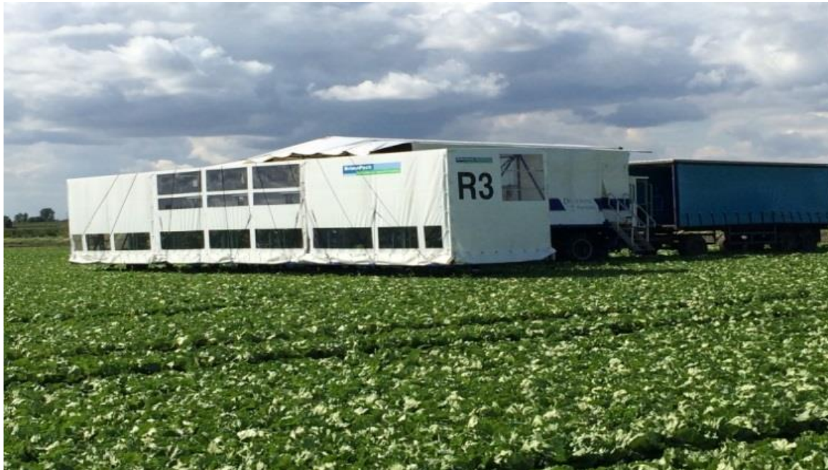
Auto wrapping lettuce harvester – 60% productivity increase
