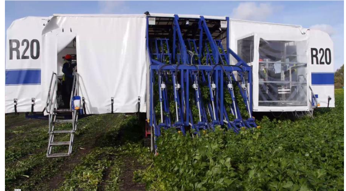
Celery auto lifting harvester – 50% productivity increase
