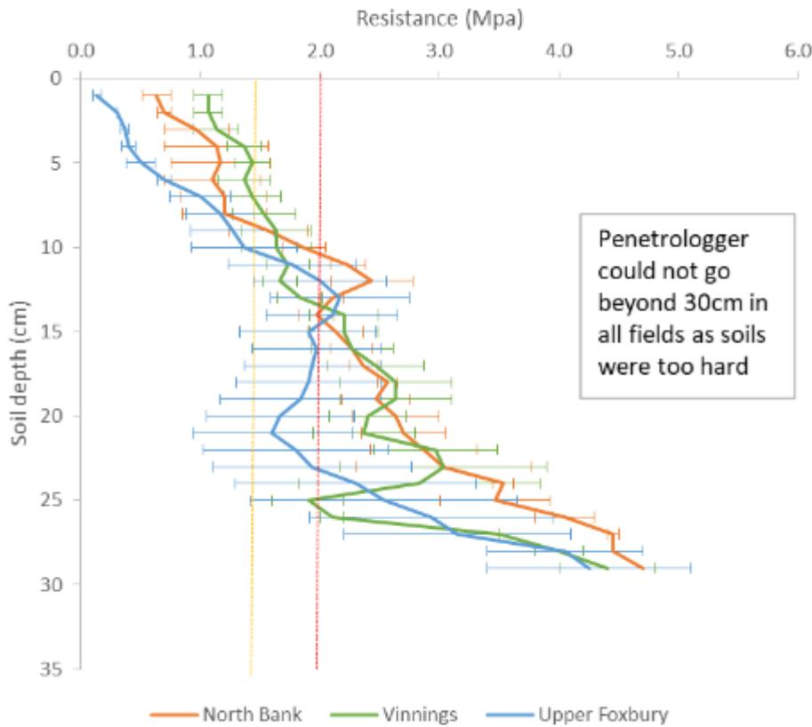
Figure 6-7 Penetration resistance profiles (December 2020); resistances >1.25 MPa indicate moderate compaction (amber dotted line) and >2 MPa high compaction with the potential to significantly impede root growth (red dotted line)
