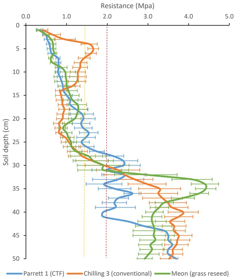
Figure 5-6 Penetration resistance profiles (November 2020); resistances >1.25 MPa indicate moderate compaction (amber dotted line) and >2MPa high compaction with the potential to significantly impede root growth (red dotted line)
