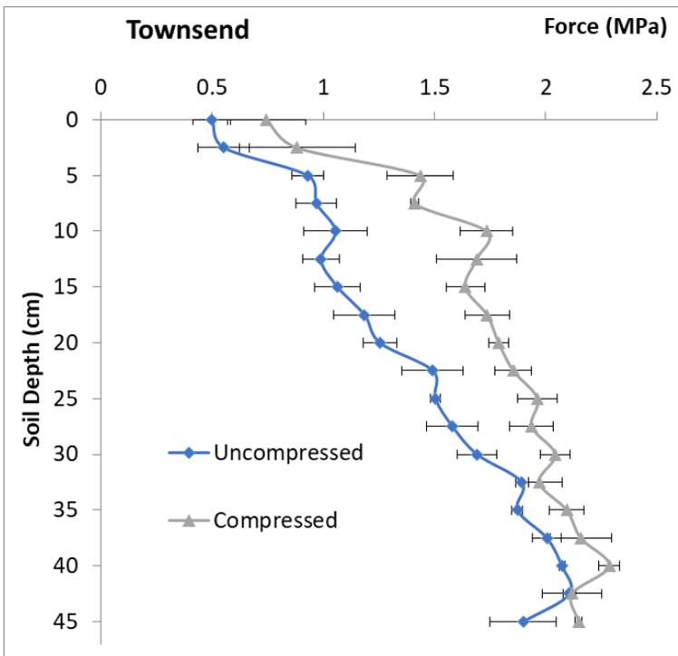
Figure 7-2 Penetration resistance profile measured in May 2020 (56.7% moisture)
