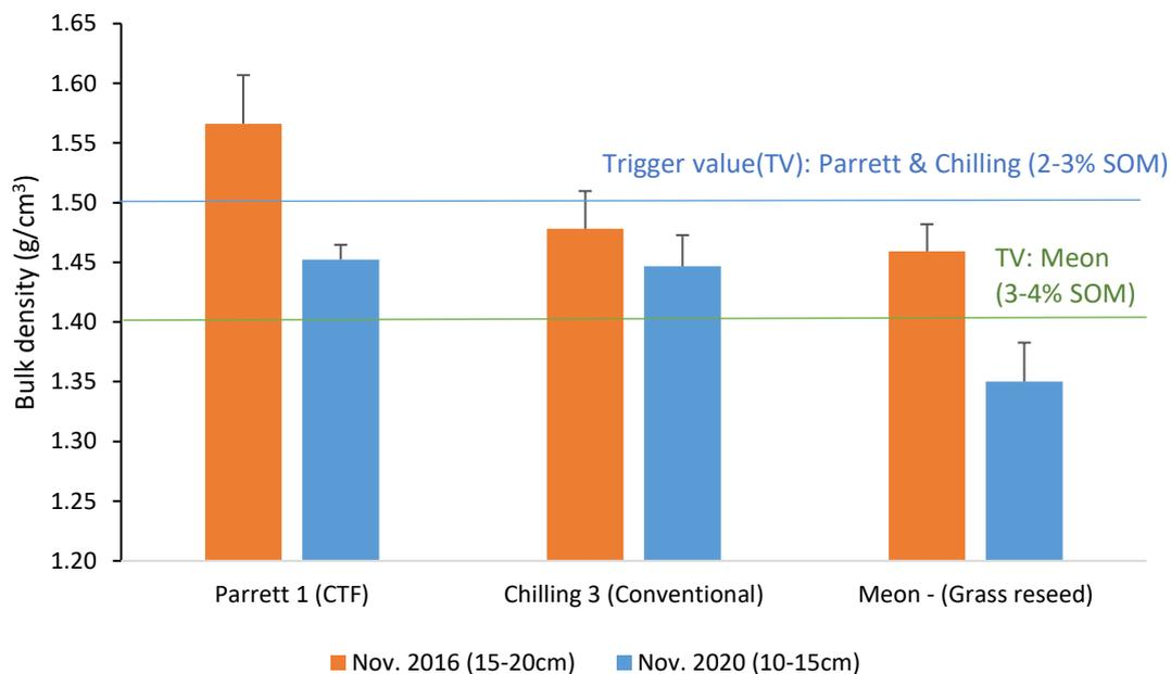
Figure 5-5 Mid-lower topsoil bulk density in 2016 and 2020, in comparison to the UKSIC Trigger values (TV).
