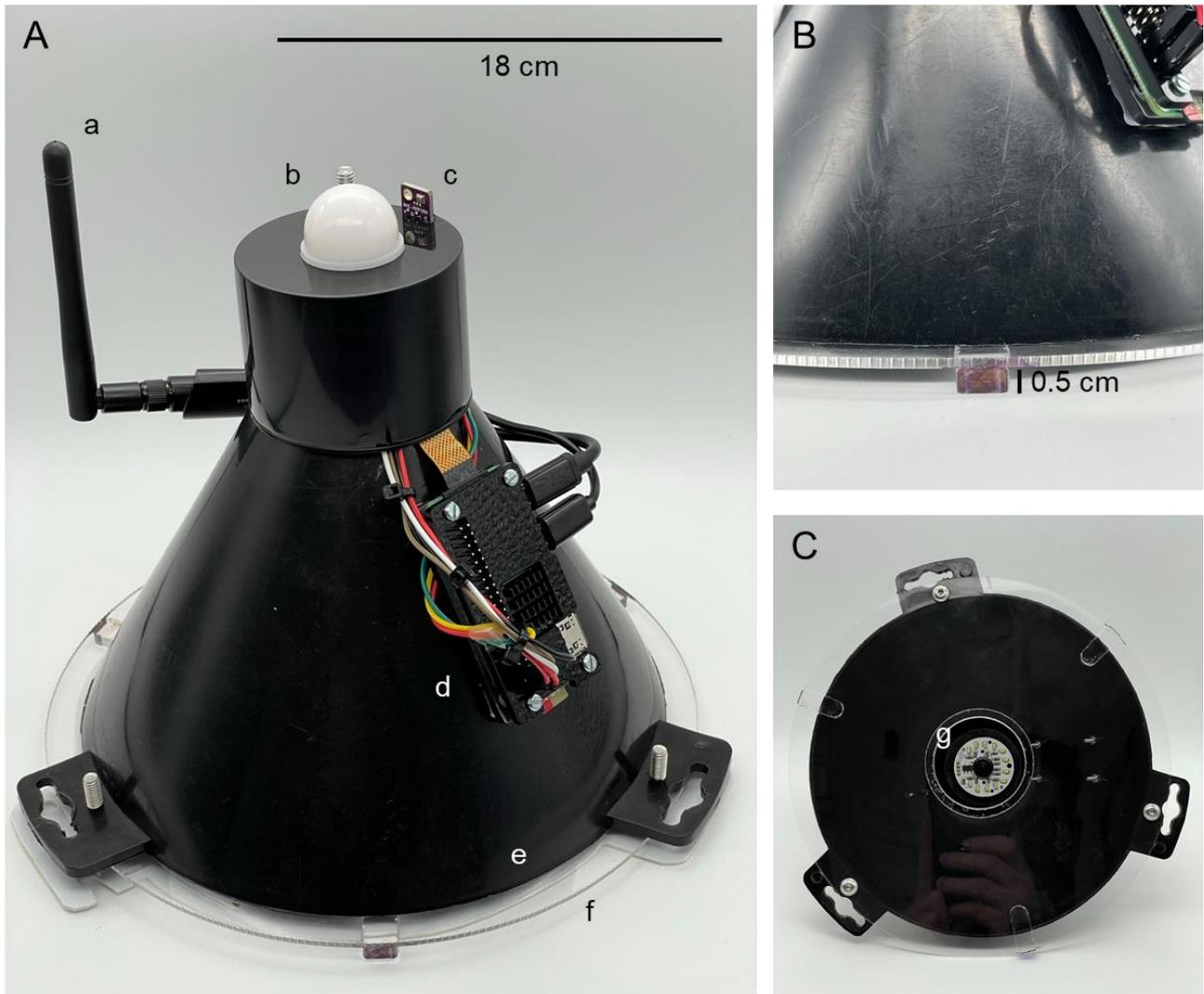
Figure 2 Modified Chemtica vine weevil trap to add smart features (A) assembled for in-field deployment with (a) Wi-Fi antenna, (b) BH1750FVI lux sensor, (c) BME280 temperature / humidity sensor, (d) Raspberry Pi
