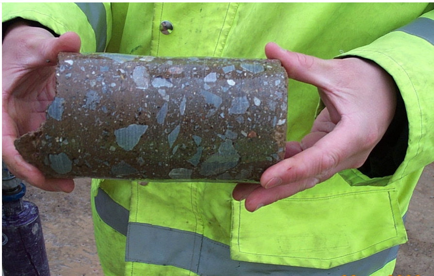
Figure 10. Example of core containing a higher percentage of aggregate
