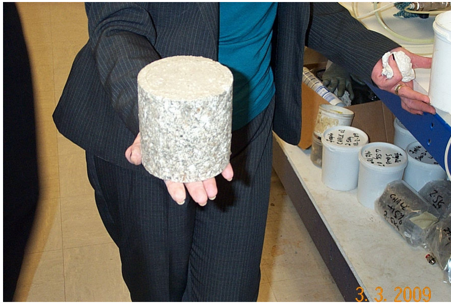
Figure 3. Compacted chalky sub-soil sample with cement inclusion
