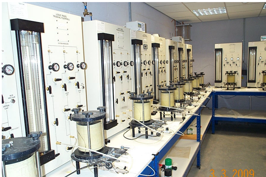
Figure 4. Sub-soil samples - Permeability testing at GeoTest laboratory
