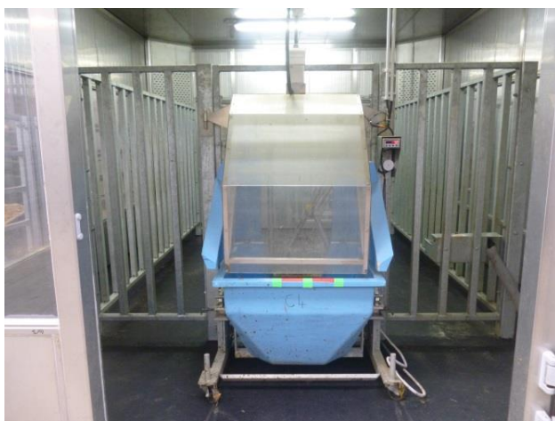
Figure 5.5a: Front view of the inside of the respiration chamber with feed intake recording equipment.
