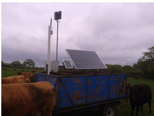
Figure 3: Trailer fitted with reader and solar panel for outdoor use at farm P
