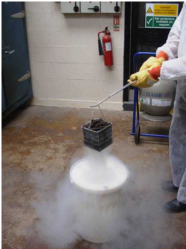
c) Lowering the sample into liquid nitrogen
