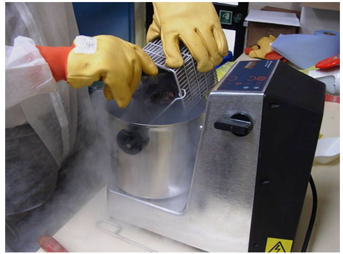
d) Transferring the sample to the homogeniser
