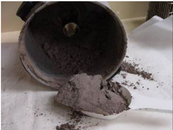
e) Typical sample after homogenisation, before thawing.
