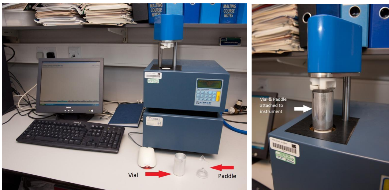
Figure 29 RVA with aluminium vial and plastic paddle on bench (left) and attached to the instrument (right).
