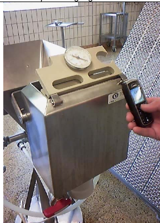
Figure 6 Knife steriliser, twin walled to improve insulation and fitted element to heat water and visual temperature gauge
